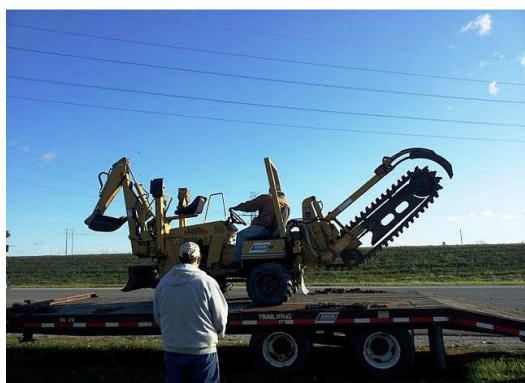
Ray Wiseman, back to camera, overseeing Tim Streit unloading a trencher provided by Newkirk Electric of Muskegon. The trencher is used to lay power lines at Muskegon's Veterans Memorial Park.
